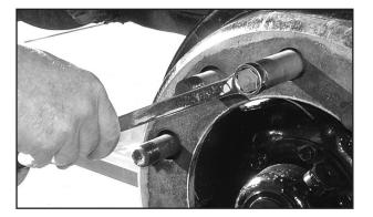
**3** Lubricate tool and install TRU-BALANCE tool at the 12, 4 and 8 o'clock positions. **DO NOT USE AN IMPACT WRENCH.**
