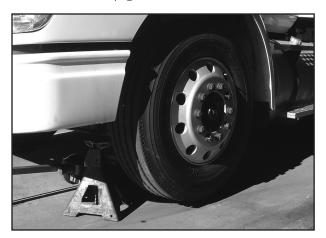
**2** Jack up the vehicle until the tire is off the ground. Always use adequate jack stands.
